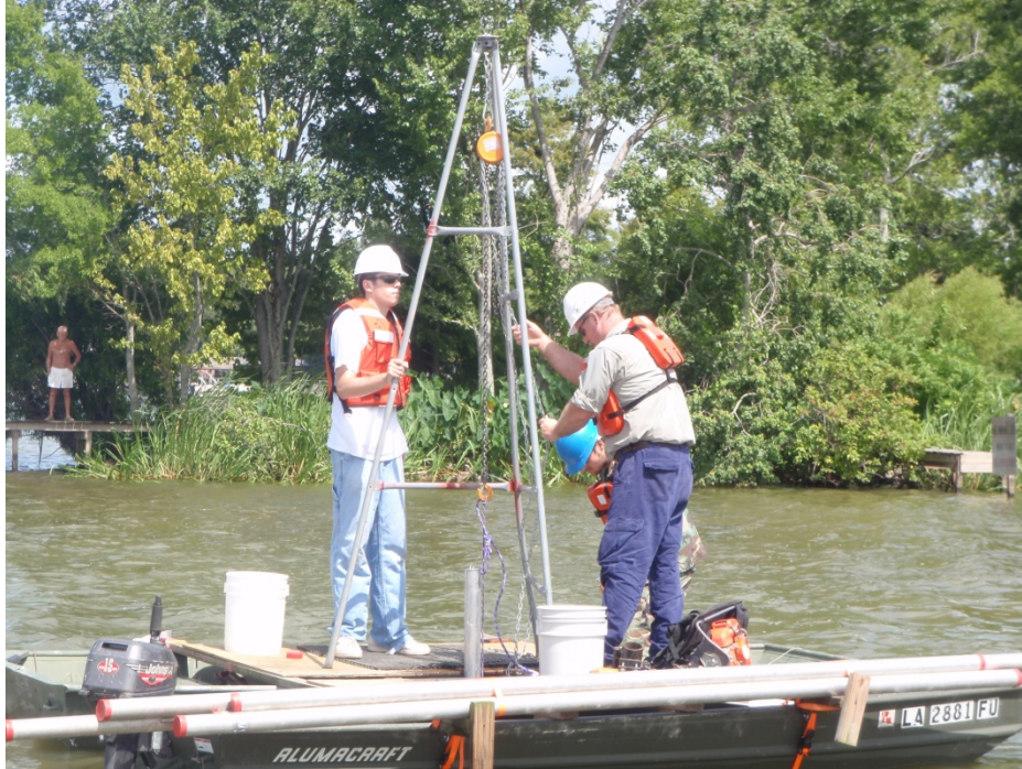
Figure 2.4. Sediment Core Sampling
